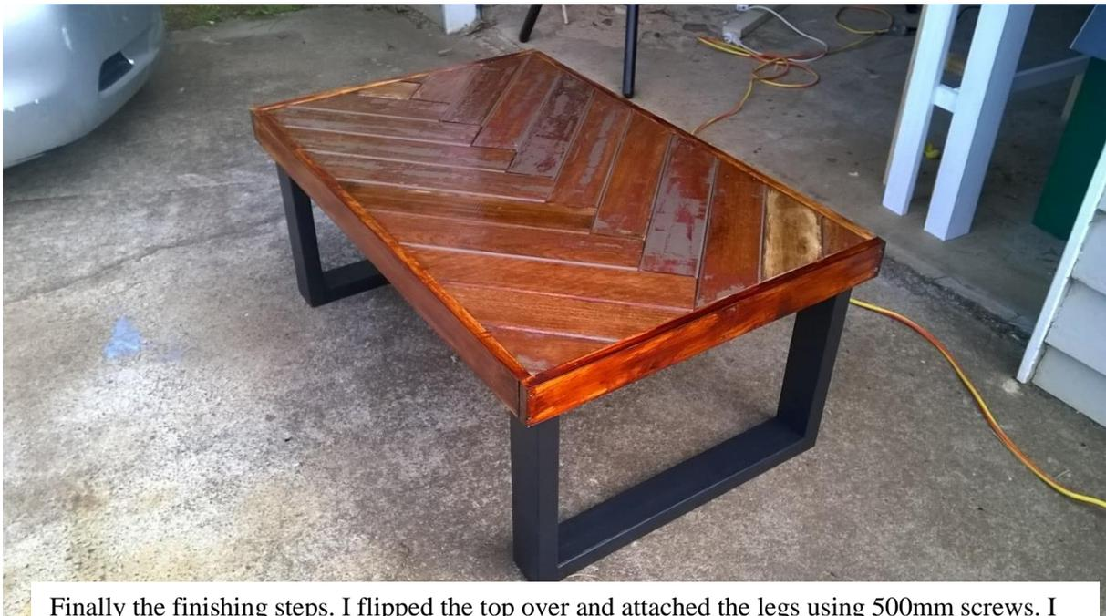
Finally the finishing steps. I flipped the top over and attached the legs using 500mm screws. I then took the table to a nice clean space free from dust and coated the top and sides with Feast Watsons Clear Varnish.
