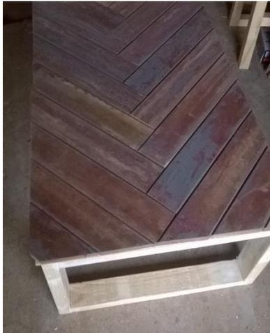
This finished top should look similar to this. I decided to reinforce the top and held another piece of ply on top and flipped it over on my workbench and drilled some 25mm screws into the back.
