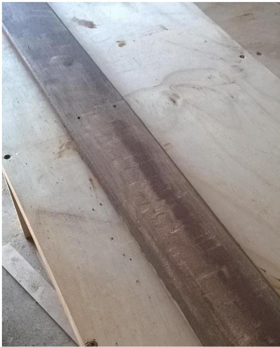
Next I sanded back each of the pieces of timber. I wanted to keep them looking rustic so I sanded each piece differently. As they were recycled I used this time to also sand back the paint drips on the side and any wear and tear on the underside to ensure a flush finish.
