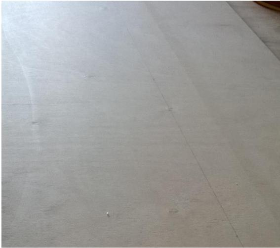
Firstly place the ply on your table and measure to ensure it's the correct length. I didn't have enough recycled timber to make the whole 1200x600 so I made mine 1180 x 600 but if you can source more recycled timber save yourself the cut and do the whole piece. I found the centre of the piece and drew a straight line down the centre.
