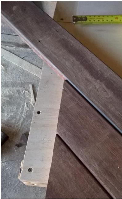
Continue this process working left and right around the table. At this stage because I don't have a nailing gun I chose to apply liquid nails and clamp as I go to save time and because I had a serious lack of clamps to work with.
